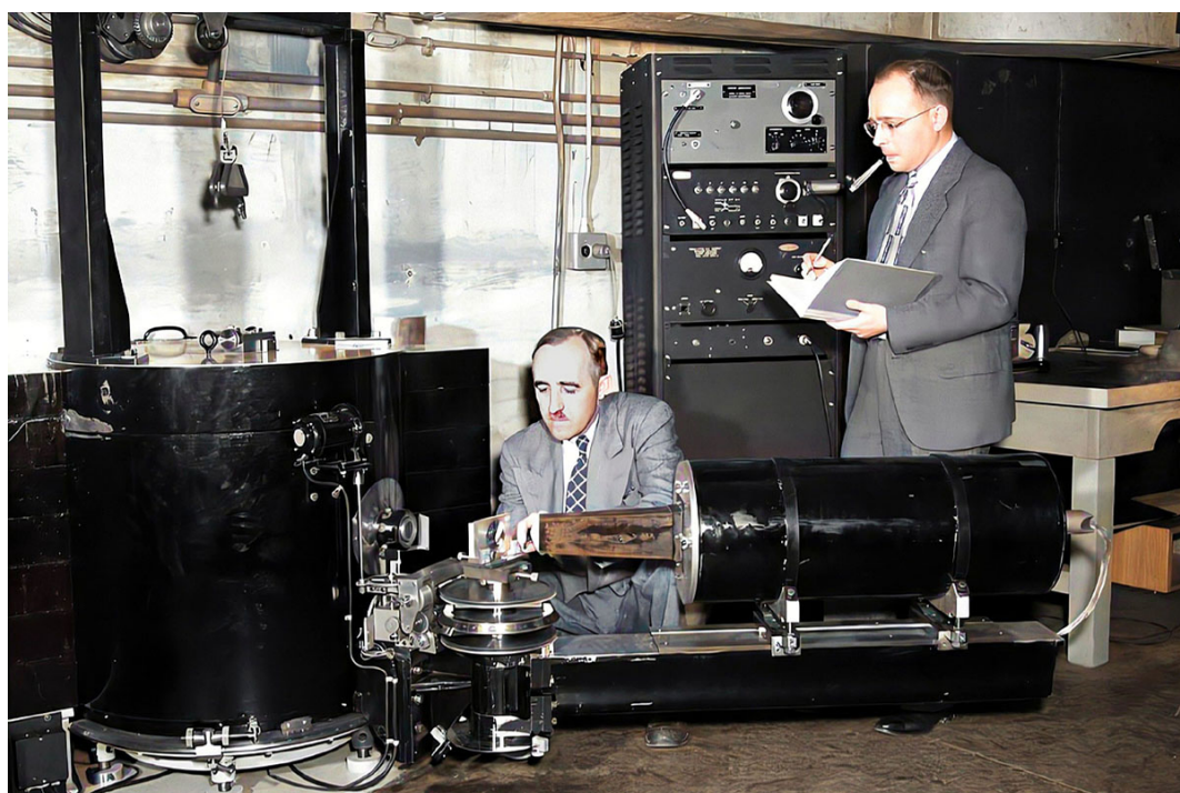
Ernest O. Wollan (kneeling) and Clifford G. Shull at the double-crystal neutron spectrometer installed at the Oak Ridge graphite reactor in 1949 (courtesy of Oak Ridge National Laboratory).
