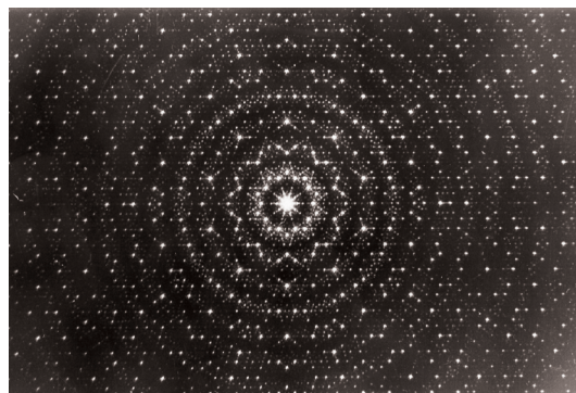
Figure 7. Simulated "electron diffraction pattern of three-dimensional Penrose tiling" in 1982, prepared for Professor Alan L. Mackay by Dr. G. Harburn at Cardiff University; courtesy of Alan Mackay, London. Used with permission.
